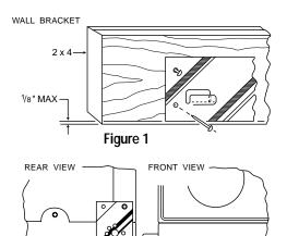
This kit consists of the following: 1 Wall mounting bracket 2 Bottom Brackets 6-1/4 x 3 inch wood screws 7-1/4 x 1-1/2 inch wood screws 12 washers
